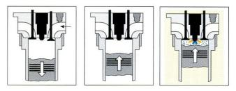
Fig. 6 Schematic drawing of direct dual-fuel injection engine work (reproduced from [9])
