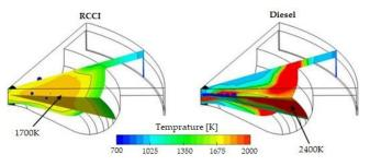
Fig. 8. Temperature distribution in the combustion chamber for a RCCI engine powered by CNG and diesel and a classic diesel engine powered only by diesel (modified graphic based on [7])
