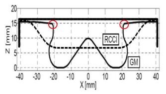
Fig. 13. Cross-section drawing of GM stock piston (solid line) and modified RCCI piston (dotted line) (reproduced from [6])
