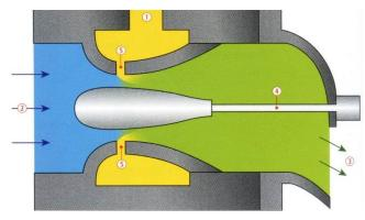
Fig. 19. A cross-sectional view of a gas mixer with an adjustable venturi insert, where 1 is the gaseous fuel supply, 2 is the air supply, 3 is the air-fuel mixture to the intake manifold of the gas- or dual-fuel engine, 4 is the adjustable venturi insert shaft connected to stepper motor, and 5 are bores for the supply of fuel-gas in the throat of the gas mixer (reproduced from [9])
