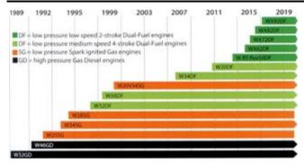
Fig. 24. Example of gaseous fuel engines development in Wärtsilä company between 1989 to 2015+ is the extensive portfolio of Wärtsilä gas- and dual-fuel engines for both two-stroke and four-stroke engine (reproduced from [9])
