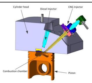
Fig. 22. The localization of the injector in CAD drawing of the cylinder head on the left and a custom gaseous-fuel injector with a parts of it on the right (reproduced from [14])
