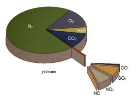
Fig. 1. The typical composition of exhaust gases from the modern, marine diesel engine (reproduced from [9])
