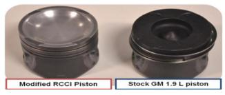
Fig. 14. Photo of modified RCCI piston and stock GM 1.9 L piston (reproduced from [1])
